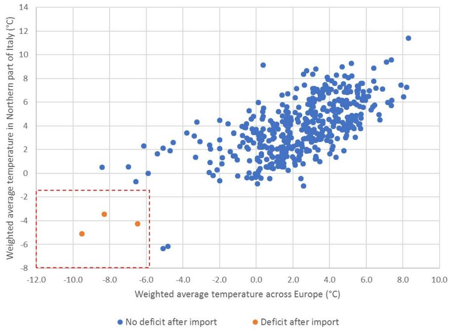
**Figure 9. Impact of daily average temperatures in Europe and in Northern Italy region for adequacy situation in Northern Italy region.**
